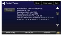
Testing Source's Response to an EDID – Provision 780's HDMI Input port with EDID from any display. Verify source responds properly to EDID. Load EDID from multiple stored EDIDs.
